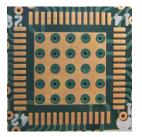
Here is a real-world example of technique B, from above. This is for a 9mm X 9mm QFN on a board using an ENIG (Electroless Nickel Immersion Gold) finish. The larger size of this part gives a little more flexibility than some of the real small parts. In this case, while the vias are left open, the area around the vias is masked to keep solder away.
