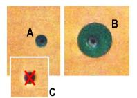
In example B, the via is capped with a wide solder mask circle. This is a decent method for non-critical applications. It is easier
