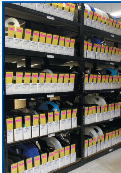
FIGURE 2: Today, direct-kitting removes boxes of parts from the line, reducing inventory to only the quantities necessary in the form of the supermarket.
