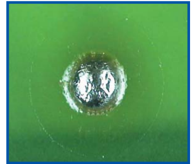
FIGURE 5: The qualified paste shows good coalescence.
