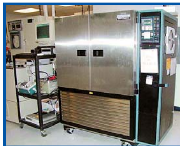
FIGURE 2: An example of a humidity chamber.
