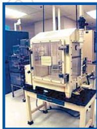
FIGURE 1: An example of a salt fog chamber.
