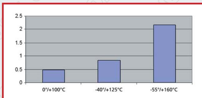
**FIGURE 3:** Normalized fatigue life for Sn63Pb37 relative to SnAg, different cycling regimes.
