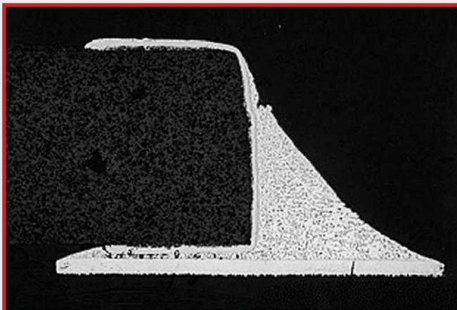
**FIGURE 1:** Microsectioned SnAgCu solder joint (after 1,000 cycles between  $-25^{\circ}/+125^{\circ}\text{C}$ ) showing fracture initiating in solder beneath the component and extending through the solder fillet.
