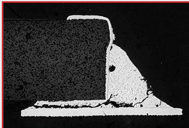
**FIGURE 2:** SnAgCu solder joint after 2,000 cycles, showing same failure mode as Pb-free joint in Figure 1.
