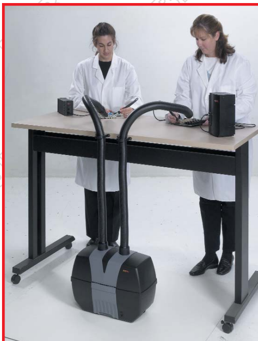
FIGURE 2: Fume extractors that can be set on the floor increase operator workspace.
