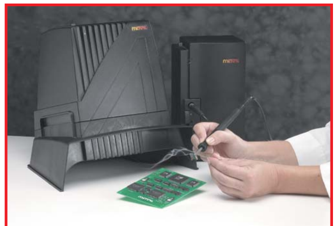
FIGURE 1: Nozzles on filtration units are positioned close to the fume source, a more efficient way of capturing airborne contaminants.
