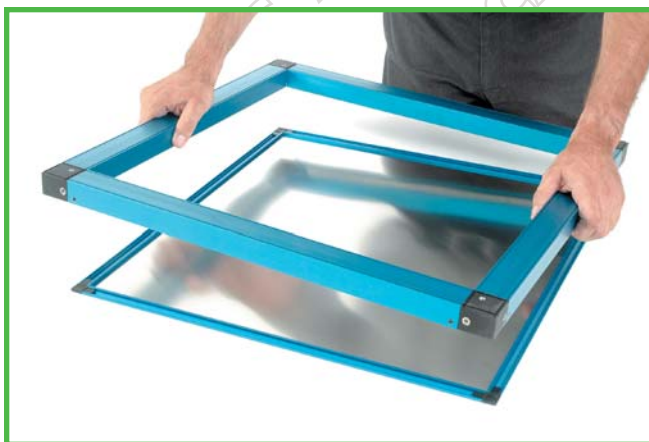
FIGURE 1: For set-up, the stencil is placed in a loading base and tensioned on the frame.
