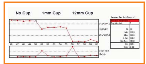
FIGURE 2: The effects of different-sized vacuum cups on the thermal signature.
