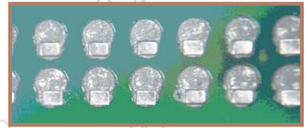
FIGURE 7: Placing rectangular segments near the through hole.
