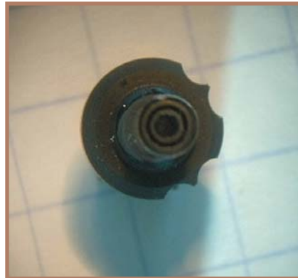
FIGURE 3: A preform washer can be placed using a nozzle that picks up the washer.
