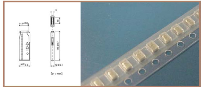
FIGURE 6: A common preform placement process is to supply the preforms using pick-and-place equipment. Paste is printed onto the through holes and the surrounding plated pads. Preforms are supplied on a tape-and-reel package or via a bulk feeder system
