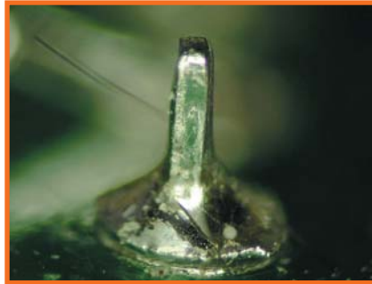
FIGURE 2: Dry joint; Sn-Ag solder, 8W. 0.8 sec.
