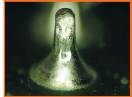
FIGURE 3: Optimized joint; Sn-Ag solder, 10W. 0.8 sec.
