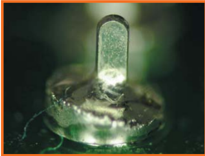
FIGURE 1: Severe dry joint; Sn-Ag solder, 6W. 0.8 sec.
