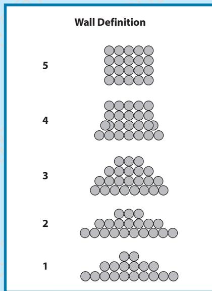
**FIGURE 1:** Solder deposit definition gauge.
